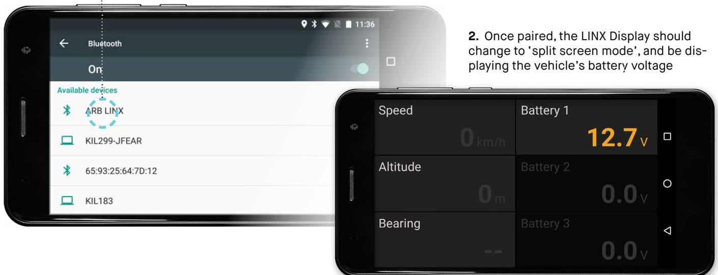
2. Once paired, the LINX Display should change to 'split screen mode', and be displaying the vehicle's battery voltage
